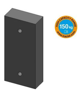
The spacer is installed with 2 chemical anchors of 12mm it is the same chemical anchor as the anchors base and does not require any specific tools.
